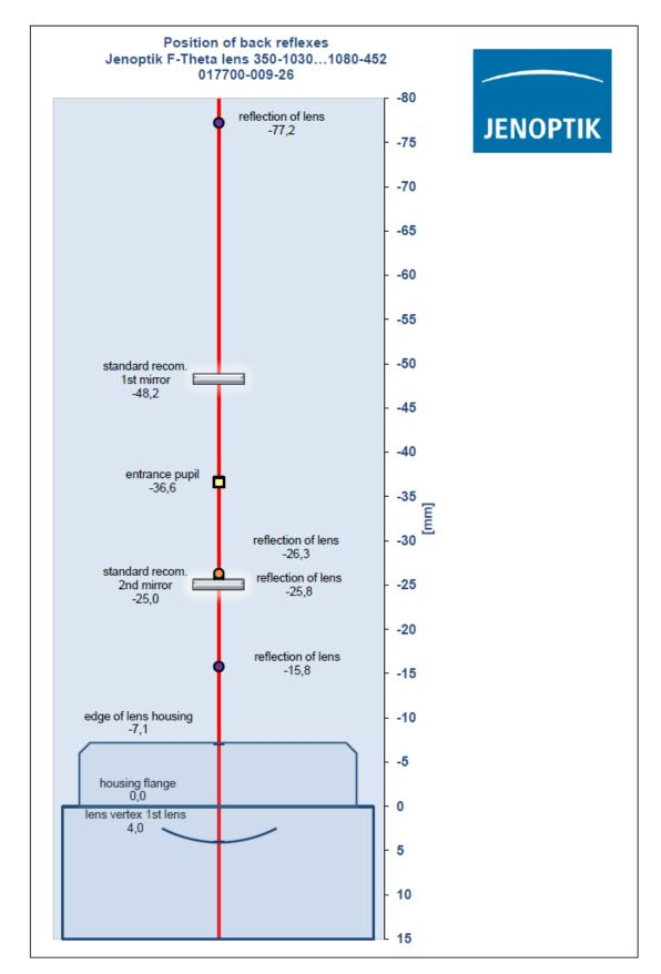
The graph illustrates all paraxial back reflection positions outside the F-Theta lens. Additional back reflection positions occur at a range of -134.5 to -210 mm and -820 mm. Back reflections inside the lens are optimized to be located away from any lens surface and element. All values are only valid for collimated beams and appropriate use of this lens. Changing system settings or operating conditions can lead to varied reflex positions and cause damage.
