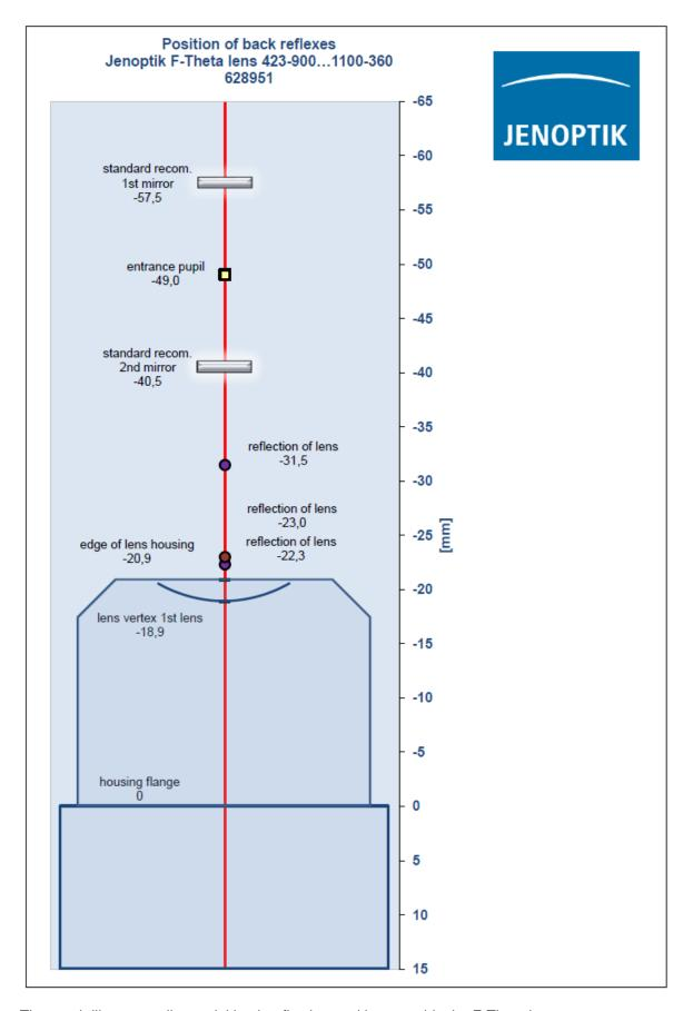
The graph illustrates all paraxial back reflection positions outside the F-Theta lens. Additional back reflection positions occur at a range of -164.1 to -164.8 mm. Back reflections inside the lens are optimized to be located away from any lens surface and element. All values are only valid for collimated beams and appropriate use of this lens. Changing system settings or operating conditions can lead to varied reflex positions and cause damage.
