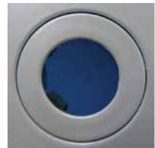
Punched with taper
